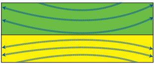
Matching corresponding sections of a polyester film roll will equalize the orientation to produce a completely flat laminated product.
