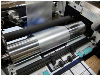
Heated Chrome Roller With High Release Silicone Nip Roller
